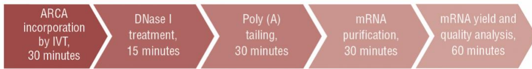
Figure 2. Overview of mRNA synthesis workflow with the HiScribe T7 ARCA mRNA Kit (with tailing)
