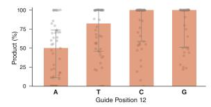
(A) Observing the reaction efficiency for a large population of randomized guides, reactions proceeded poorly when the twelfth position of the guide was adenosine.
