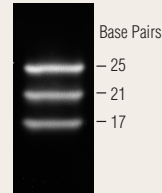
siRNA Marker (dsRNA) 45 ng/lane 20% TBE polyacrylamide gel
