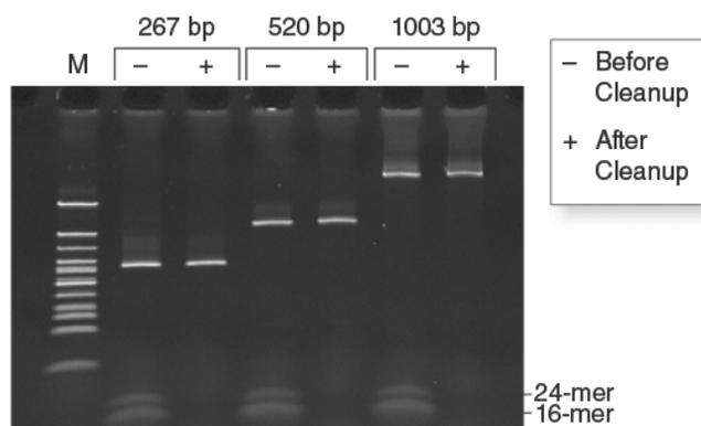
Three independent amplicons (267 bp, 520 bp, 1003 bp) were spiked with two oligonucleotides (16-mer, 24-mer) to a final concentration of 1 µM. Half of each mix was purified with the Monarch PCR & DNA Cleanup Kit (5 µg) following the included protocol. Equivalent fractions of the original mixture and the eluted material were resolved on a 20% TBE acrylamide gel at 100V for one hour and stained with SYBR Green II.
