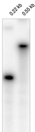
*Labeling reactions were incubated for 10 minutes at room temperature. A small portion of each reaction was run on a 6% PAGE urea gel followed by exposure of the gel to a Storage Phosphor Screen (GE).*
