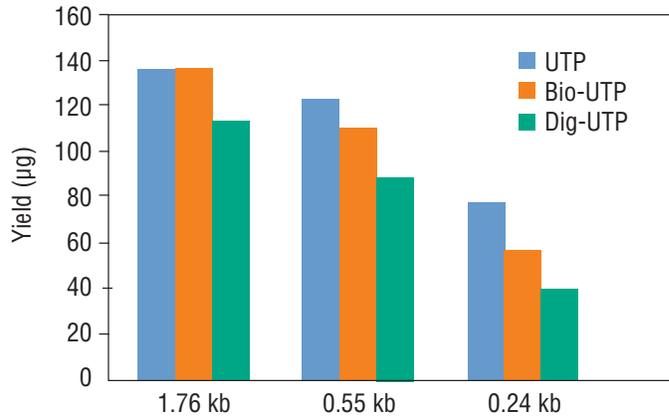
*RNA synthesis reactions using linearized plasmid DNA templates were performed in the presence of unmodified nucleotides or modified nucleotides (Biotin-UTP, Digoxigenin-UTP) at the ratio of 2.3:1 (UTP:modified UTP). Reactions were incubated at 37°C in a PCR machine for 2 hours. Transcripts were treated with DNase I, purified by LiCl precipitation and quantified using a NanoDrop Spectrophotometer.*
