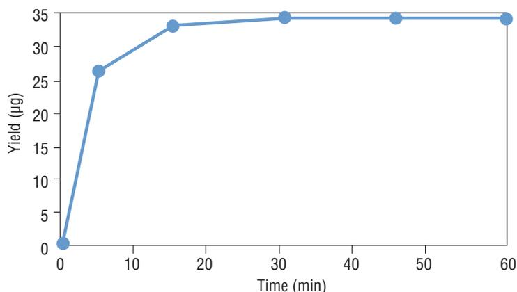
*SP6 control template (1.76 kb) was transcribed in the presence of 4 mM ARCA at 37°C in a PCR machine over one hour. Transcripts were treated with DNase I, purified by LiCl precipitation and quantified using a NanoDrop Spectrophotometer.*
