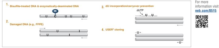
Archaeal family B-type polymerases can incorporate/tolerate a variety of modified nucleotides but will stall upon encountering uracil and inosine residues. Q5U Hot Start High-Fidelity DNA Polymerase is a modified Q5 High-Fidelity DNA polymerase which efficiently incorporates dUTP and amplifies uracil-containing templates. Common applications enabled by Q5U Hot Start High-Fidelity DNA Polymerase are illustrated above.
