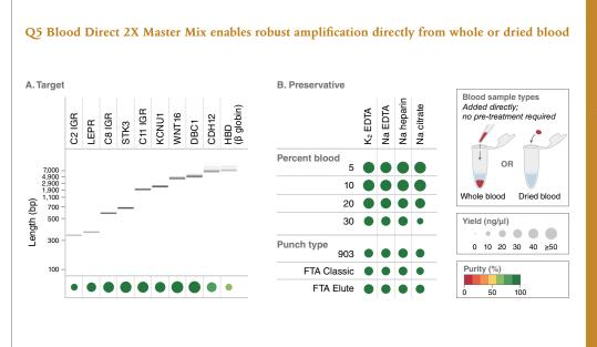
PCR was performed using Q5 Blood Direct 2X Master Mix under standard recommended conditions with 35 cycles of amplification. Yield and purity were quantitated by microfluidic LabChip® analysis and are indicated by dot size and color, respectively, with a large, dark green dot representing the strongest performance.
