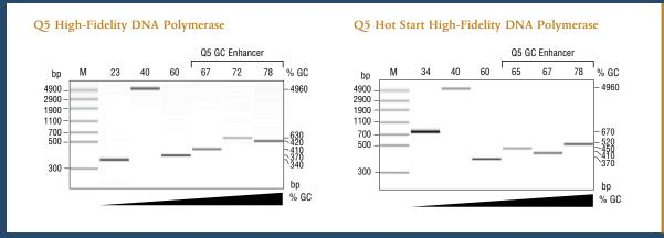
Robust amplification with 05 and 05 Hot Start High-Fidelity DNA Polymerases, regardless of GC content: Amplification of a variety of human genomic amplicons from low to high GC content using either 05 or 05 Hot Start High-Fidelity DNA Polymerase. Reactions using 05 Hot Start were set up at room temperature. All reactions were conducted using 30 cycles of amplification and visualized by microfluidic LabChip® analysis.
