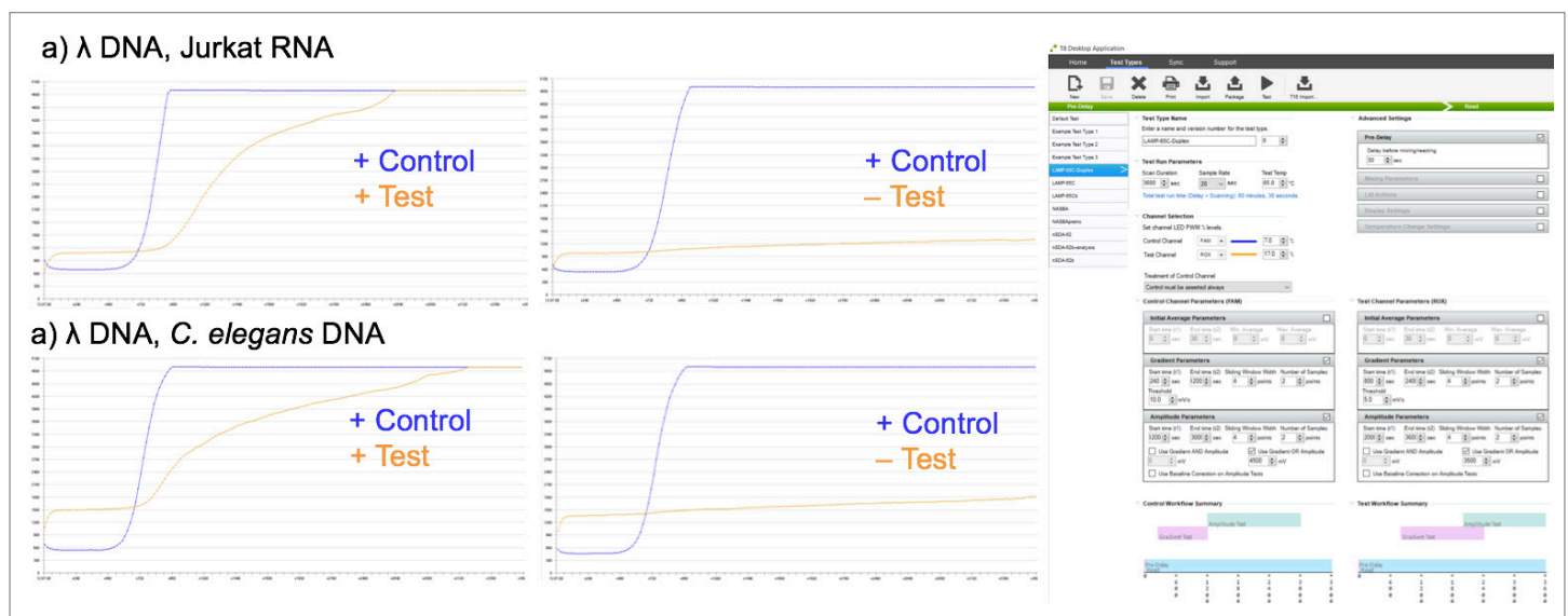
FIGURE 2: 2-plex LAMP reaction using NEB's WarmStart Colorimetric LAMP 2X Master Mix and Axxin's T8-ISO instrument, using the FAM control assay
