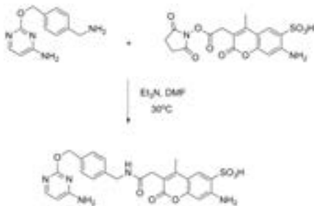
Figure 2. Coupling of BC-NH 2 to Alexa Fluor® 350 NHS ester. A solution of 2.4 mg (5.8 μmol) Alexa 350 NHS-ester in 500 μl DMF was added to 2.0 mg (8.7 μmol) BC-NH 2 and 1.2 μl triethylamine (8.7 μmol) in 500 μl DMF. The reaction was shaken at 30°C overnight. The solvent was evaporated under vacuum. The reaction was diluted in 1 ml water / acetonitrile (9:1) and the product purified by reverse phase HPLC.
