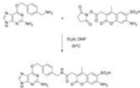
Figure 2. Coupling of BG-NH 2 to Alexa Fluor® 350 NHS ester. A solution of 2.0 mg (4.9 μmol) Alexa 350 NHS-ester in 500 μl DMF was added to 2.0 mg (7.4 μmol) BG-NH 2 and 1.1 μl triethylamine (7.9 μmol) in 500 μl DMF. The reaction was shaken at 30°C overnight. The solvent was evaporated under vacuum. The reaction was diluted in 1 ml water/acetonitrile (9:1) and the product purified by reverse phase HPLC.
