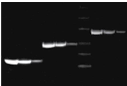
Figure 3. Typical SDS-PAGE gel under UV transillumination (Lane 1-3 SNAP-his (22kD) 10, 5, 1  $\mu$ g; Lane 4-6 SNAP-CyA (40kD) 10, 5, 1  $\mu$ g; Lane 7 fluorescent MW markers (Sigma P/N F3526-1VL); Lane 8-10 MBP-SNAP (63kD) 10, 5, 1  $\mu$ g).
