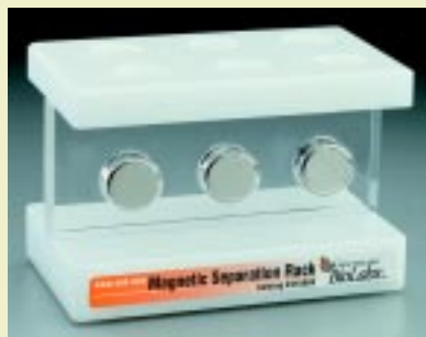
NEB's Magnetic Separation Rack holds six 1.5 ml Eppendorf tubes and, for a limited time, is supplied with free samples of Streptavidin and Protein A Magnetic Beads.
