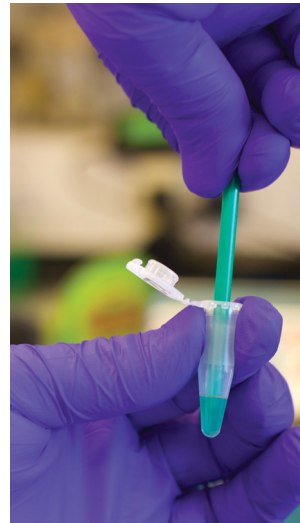
Microtube pestle and grinding tube included for optimal sample homogenization.
